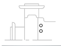
**Description:** Plan 03 is a dead-ended seal chamber with an open throat, tapered seal chamber and flow modifiers to generate product circulation.
