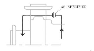
**Description:** Plan 13 is recirculation from the seal chamber or gland through an 1/8" minimum flow control orifice (when necessary), back to the pump suction. Standard flush plan for vertical pumps.
