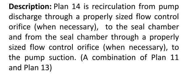
**Objective:** Remove seal generated heat and vent vertical pumps while providing adequate seal chamber pressure for process vapor margin and sufficient fluid flow for cooling.
