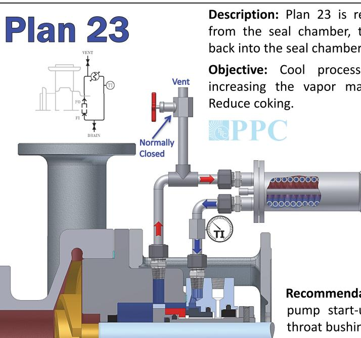
**Description:** Plan 23 is recirculation of process fluid from the seal chamber, through a seal flush cooler, back into the seal chamber utilizing a pumping ring.
