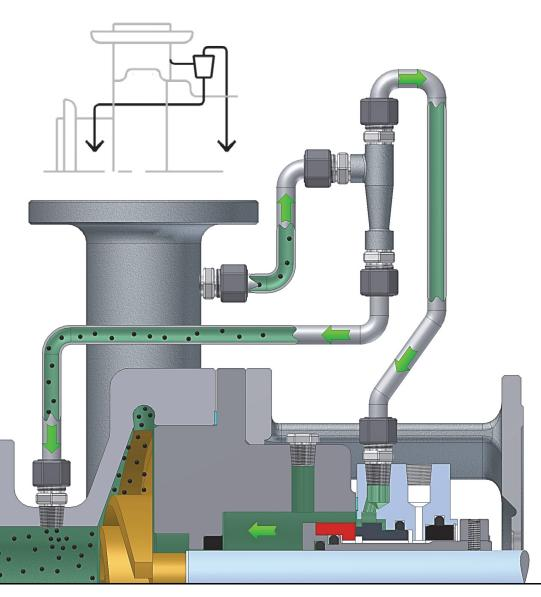
**Description:** Plan 31 is recirculation from pump discharge through a CYCLONE SEPARATOR, sending clean flush into the seal chamber and heavy particles back to pump suction.
