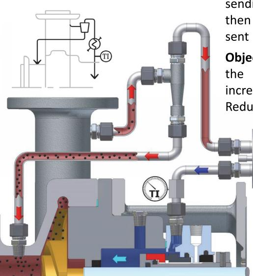
**Description:** Plan 41 is recirculation from pump discharge through a CYCLONE SEPARATOR, sending clean flush through a seal flush cooler, then into the seal chamber. Heavy particles are sent back to pump suction.
