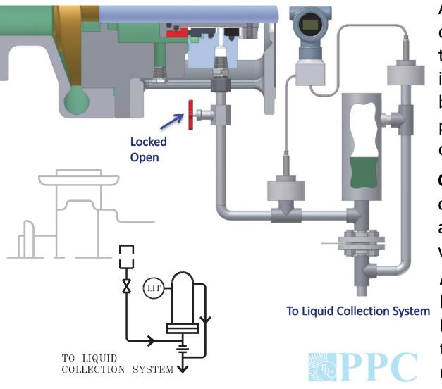
Arrangement 1 single seals. The orifice downstream of the level transmitter is typically 1/4" located in a vertical piping leg. Includes a bypass around the orifice to prevent pressure build up. Use with close-clearance gland throttle bushing.
