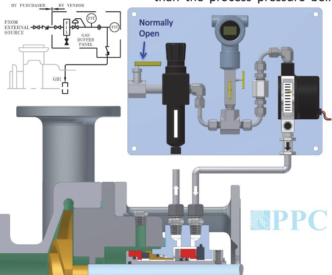
dual gas seal, with a dry running containment seal. Used alone to dilute seal leakage or in conjunction with Plan 75 or 76 to help sweep seal leakage into a closed collection system.
