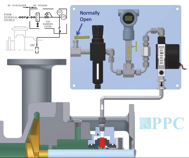
Objective: Prevent process from leaking to the atmosphere. Remove moisture, filter the gas and regulate the pressure to the seal. Best for hazardous, non-polymerizing, non-oxidizing fluids, light hydrocarbons and vapors.
