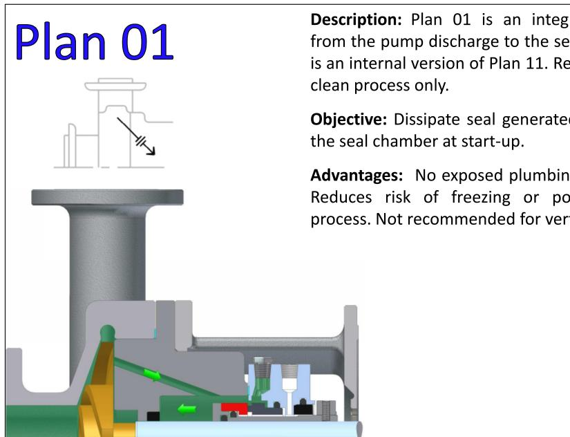
**Description:** Plan 01 is an integral recirculation from the pump discharge to the seal chamber. This is an internal version of Plan 11. Recommended for
