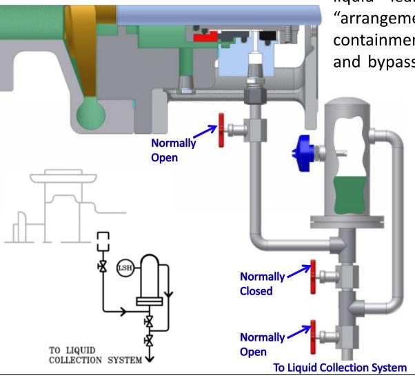
Description: Plan 65B is a TOTAL liquid leakage detection system measuring accumulated liquid leakage. Normally for single seals "arrangement 1". Seal leakage will collect in a containment vessel with a high level switch and bypass line to prevent pressure build up.
