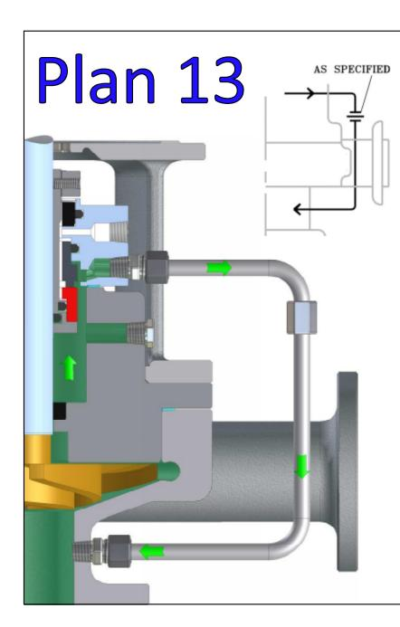
**Description:** Plan 13 is recirculation from the seal chamber or gland through an 1/8" minimum flow control orifice, when necessary, back to the pump suction. Is a standard flush plan for vertical pumps.
