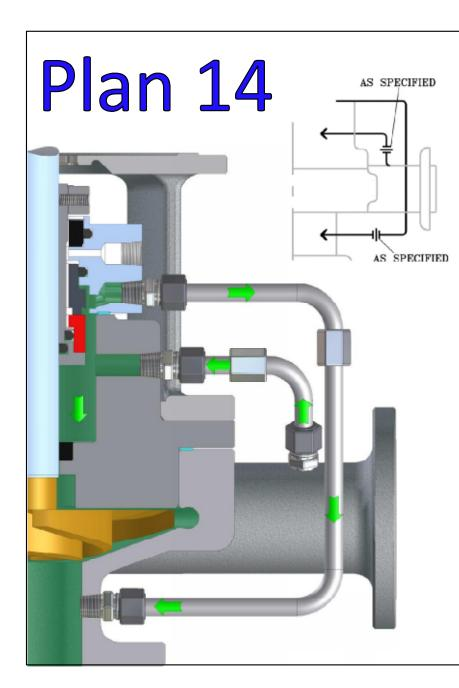
**Description:** Plan 14 is recirculation from pump discharge through a properly sized flow control orifice, when necessary, to the seal chamber and from the seal chamber through a properly sized flow control orifice, when necessary, to the pump suction. (A combination of Plan 11 and Plan 13)
