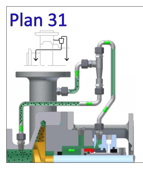
**Description:** Plan 31 is recirculation from pump discharge through a CYCLONE SEPARATOR, sending clean flush into the seal chamber and heavy particles back to pump suction.
