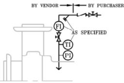
**Objective:** Isolate fluid in the seal chamber from process. Using a close clearance throat bushing, the injected fluid can isolate the seal from a process with poor lubricity, high temperature, abrasive, dirty, corrosive, polymerizing, or oxidizing properties. To provide cooling to the seal.
