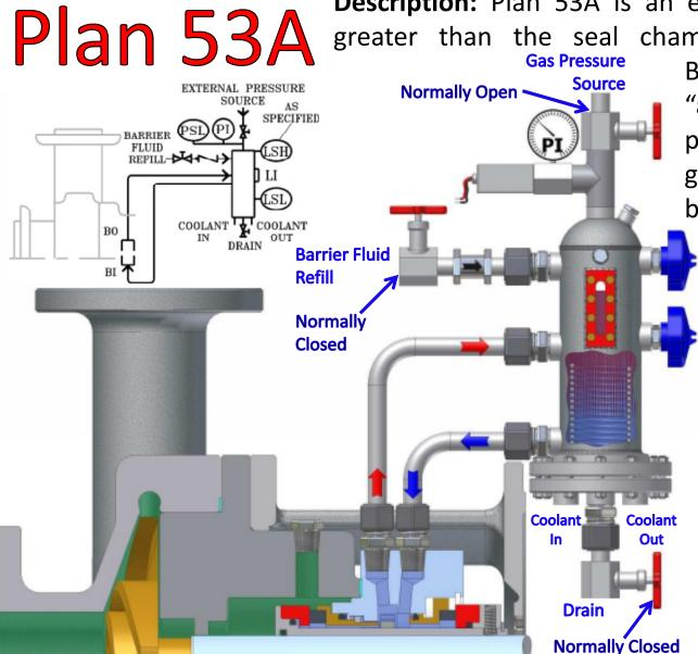
**Description:** Plan 53A is an external reservoir, PRESSURIZED greater than the seal chamber pressure. Provides clean
