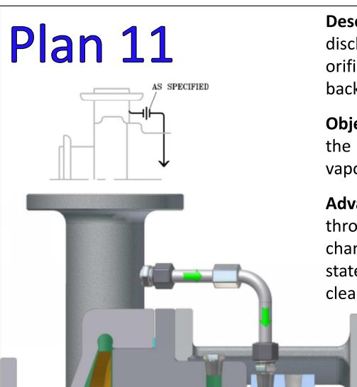
**Description:** Plan 11 is recirculation from pump discharge through an 1/8" minimum flow control orifice, when necessary, to the seal and flows back into the pump.
