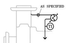
**Description:** Plan 21 is recirculation from pump discharge through an 1/8" minimum flow control orifice, when necessary, and seal flush cooler, then into the seal chamber.
