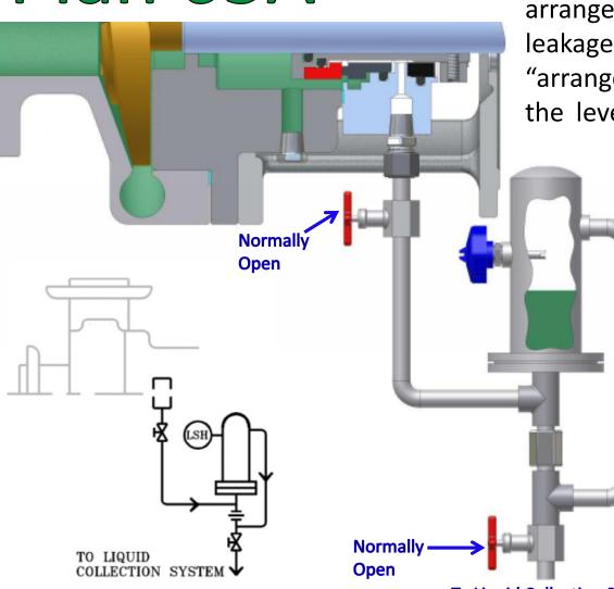
**Description:** Plan 65A is a liquid leakage detection system measured by a level switch, arranged to set off an alarm when EXCESSIVE leakage occurs. Normally for single seals "arrangement 1". The orifice downstream of the level switch is typically 1/4" located in a
