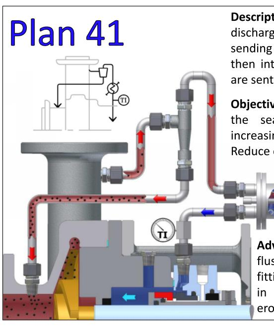
**Description:** Plan 41 is recirculation from pump discharge through a CYCLONE SEPARATOR, sending clean flush through a seal flush cooler, then into the seal chamber and heavy particles are sent back to pump suction.
