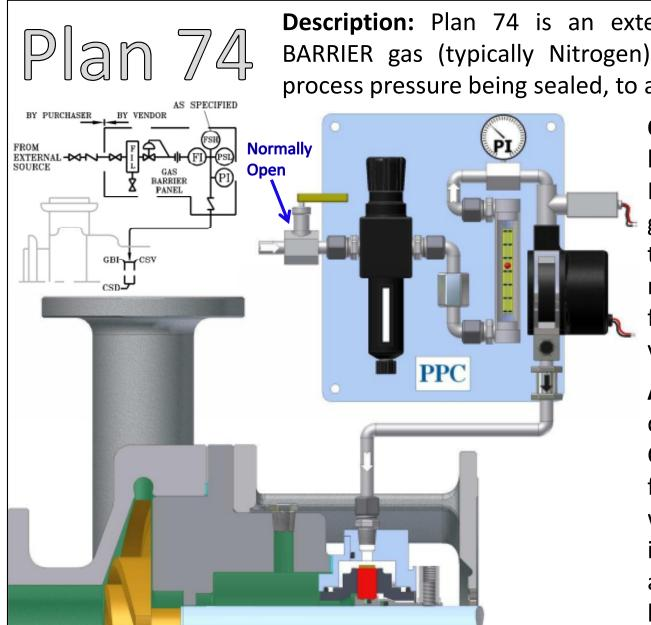
**Description:** Plan 74 is an external control system supplying BARRIER gas (typically Nitrogen) at greater pressure than the process pressure being sealed, to a dual gas seal "arrangement 3".
