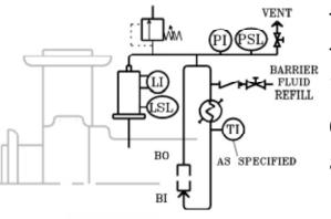
**Description:** Plan 53C utilizes a reference line from the process in the seal chamber as a pressure source to a PISTON ACCUMULATOR. Provides a PRESSURIZED system greater than the process pressure being sealed, providing clean BARRIER fluid to a dual seal "arrangement 3". Circulation is by an internal pumping ring.
