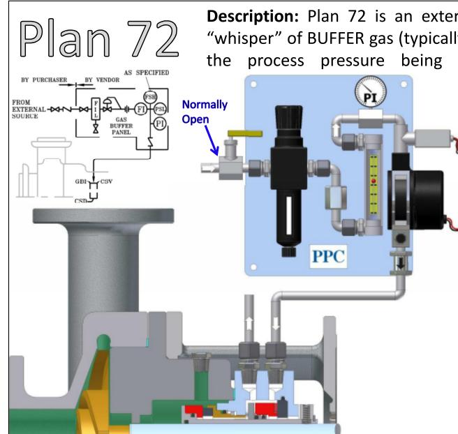
**Description:** Plan 72 is an external control system supplying a "whisper" of BUFFER gas (typically Nitrogen) at less pressure than the process pressure being sealed, to a dual gas seal
