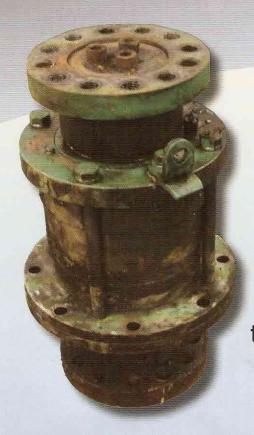
A complete seal assembly, including a stub shaft, is routine work for PPC. The seals are completely disassembled, cleaned and inspected. PPC will evaluate all critical tolerances and fits to insure "like new" condition of the complete assembly.
