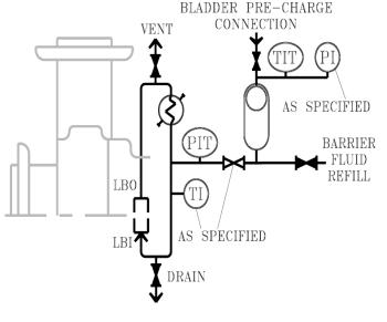
**Description:** Plan 53B utilizes a pre-pressurized BLADDER ACCUMULATOR isolating pressurized gas from barrier fluid and providing a PRESSURIZED system greater than the process pressure being sealed. Provides clean BARRIER fluid to an Arrangement 3 dual seal. Circulation provided by an internal pumping ring.
